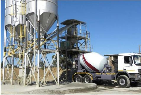
The Readymix division supplies concrete primarily to large-scale civil engineering and infrastructure projects through fixed and mobile readymix plants where concrete is batched on demand and then transported to site by concrete mixer trucks. Close to 90% of Readymix's raw material needs (excluding cement) are sourced from the group's own quarries.
